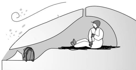
Figure 8.9: Creating ventilation in a snow tunnel
