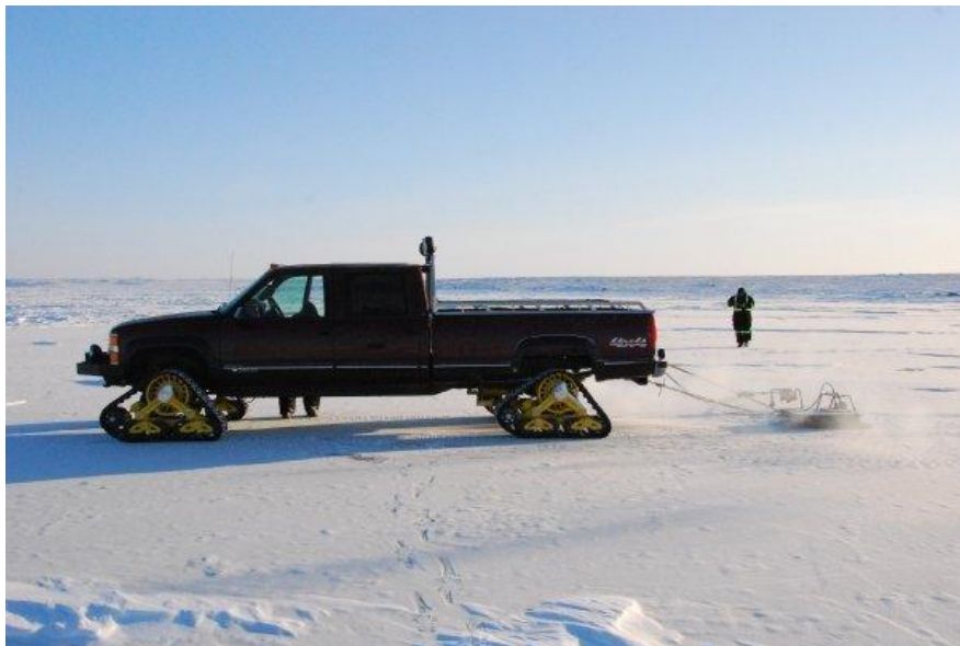
Figure 21.3: Light truck with track conversion towing ground penetrating radar (GPR) ice profiling equipment © Iain Mitchell
