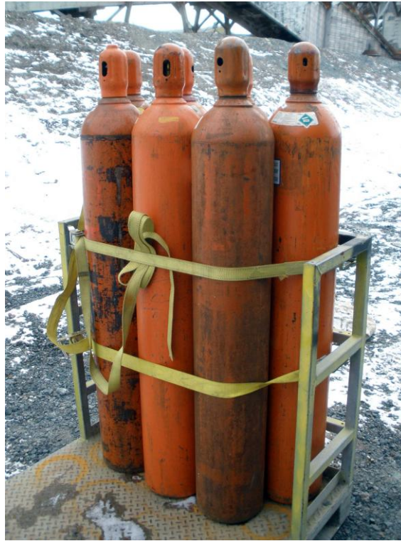
Figure 18.6: Correctly stored compressed gas cylinders – upright, secured with safety caps in place and off wet ground to prevent corrosion. © Courtney Mitchell
