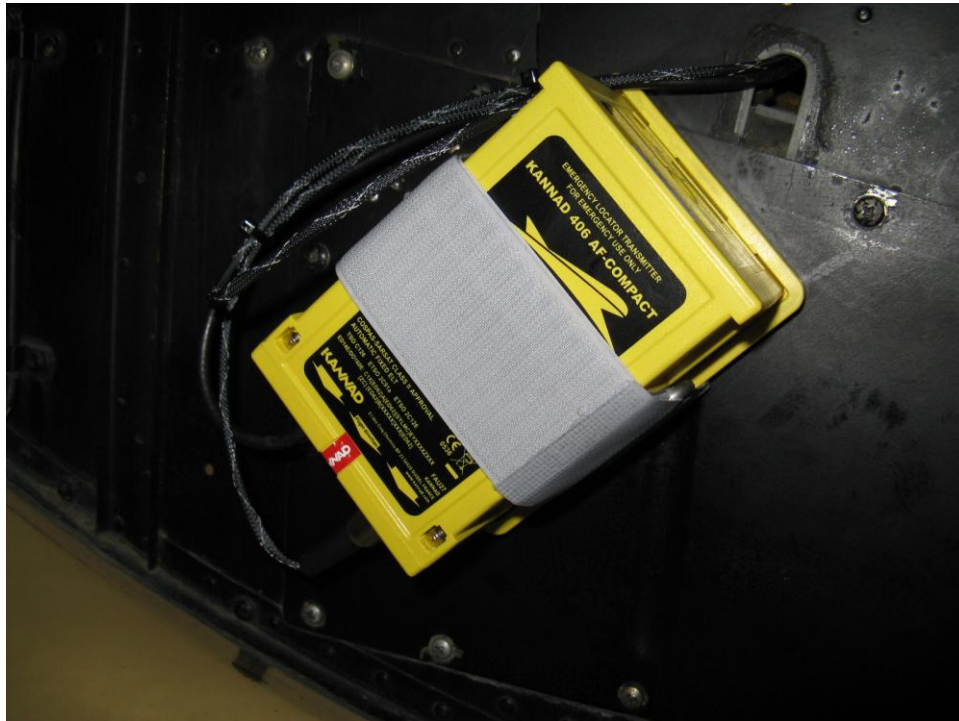
Figure 7.1: 406 MHz Emergency Locator Transmitter (ELT) mounted in a helicopter. Know the location and how to manually activate the ELT whenever you fly in charter aircraft. © Great Slave Helicopters
