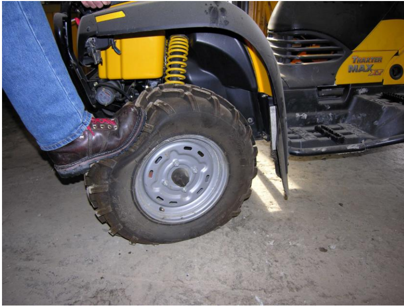
Figure 14.1: Check the tire pressure before setting out each day. Carry a low pressure tire gauge and a tire pump. © Courtney Mitchell
