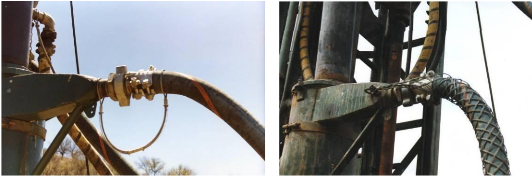
Figure 20.5: Standard whip check (left) and cable stocking whip check (right) © Bill Mitchell
