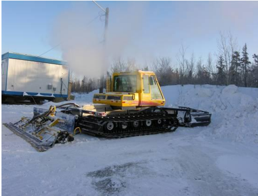
Figure 21.4: Wide tracked Sno-cats are used to clear ice roads and runways on ice. © Iain Mitchell
