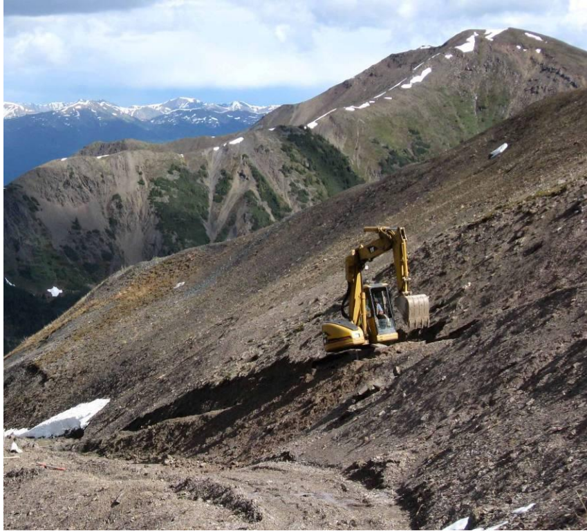
Figure 21.1: Do not stand or work downhill from heavy equipment in case it rolls or knock debris downhill. © Matt Turner
