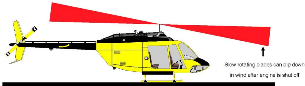
Figure 16.4: Helicopter blades can dip down in wind
