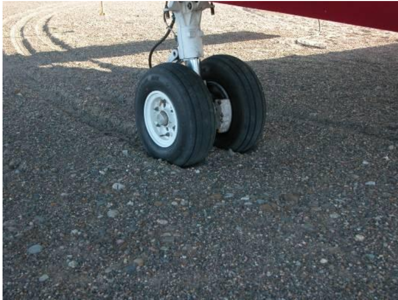
Figure 16.10: Try to verify the condition of a remote landing strip; this aircraft had to be towed to firmer ground before departure. © Bill Mitchell
