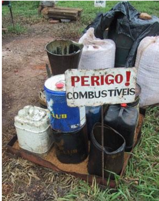
Figure 40: On this drill site in Brazil, combustible fluids are stored separately on a metal pan filled with sawdust to absorb any inadvertent drips or spills. The sawdust can be disposed of safely at the end of the program. © Servitec.
