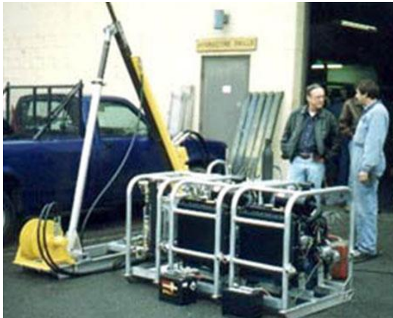
Figure 64: Modular rig ready for mobilization to the project. © Kluane Drilling.
