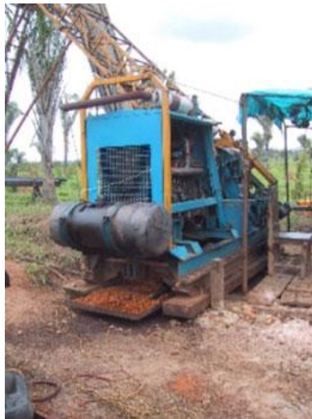
Figure 41: Note the pan filled with wood chips underneath the rig on this drill site in Brazil. Inadvertent drips and spills are absorbed by the wood chips and can be disposed of safely. © Servitec.
