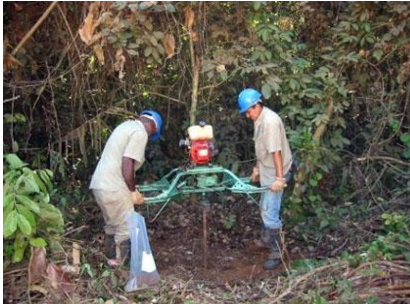
Figure 67: Preliminary exploration (auger drilling) in the rain forests of Carajas, Brazil. © Noranda/Falconbridge.
