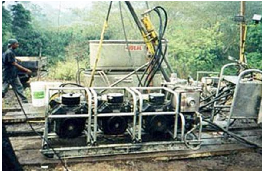
Figure 65: Drill rig showing three tandem engines for increased portability with no loss of power. © Kluane Drilling.
