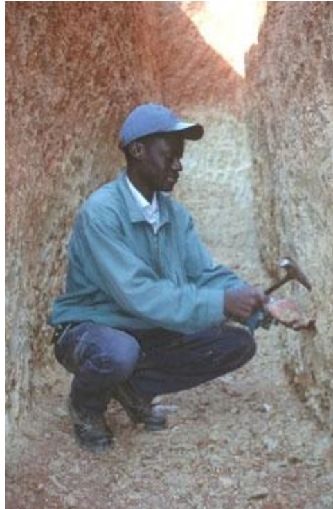
Figure 36: Deep trenches are often required in tropical to semi-tropical terrain to assess saprolitic deposits. If used, project managers must seriously address issues of safety for the workers. © lamgold.
