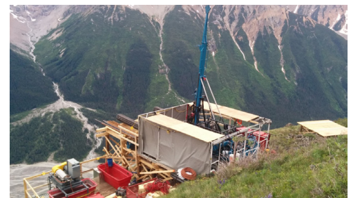
HY-TECH drill with plug in centrifuge system, on site in NW British Columbia.
