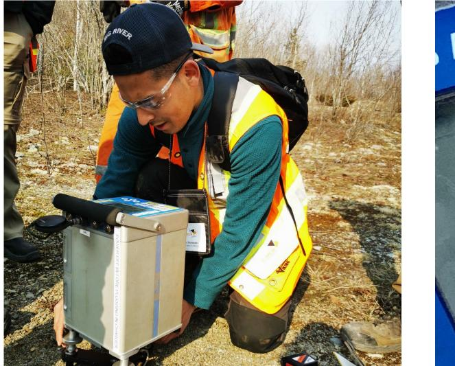
Billy (University of Victoria) levelling the gravitometer for a gravity survey.
