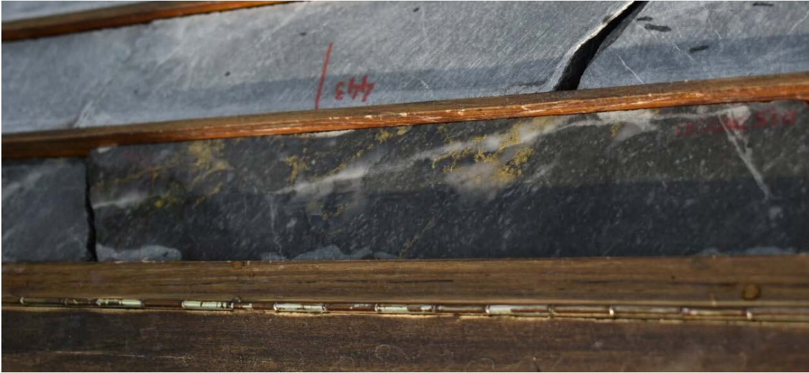
Figure 4. Visible gold in diamond drill core at North Mara Gold Mine
