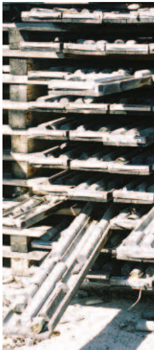
Drill core samples spilling out of boxes are often found at abandoned exploration sites
