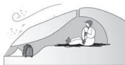
Snow tunnel with air holes
